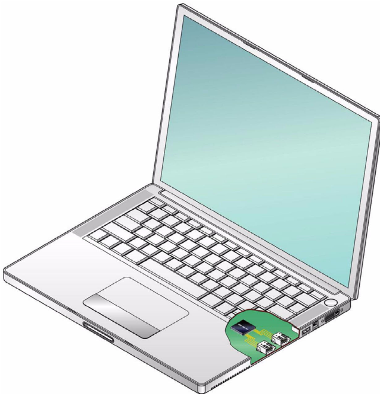
Figure 9-1—Overview of notebook computer showing implementation of IEEE 1394 ports.
