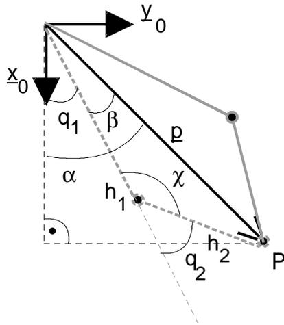
**Figure 3-4:** Geometrical solution of 2 dof robot
