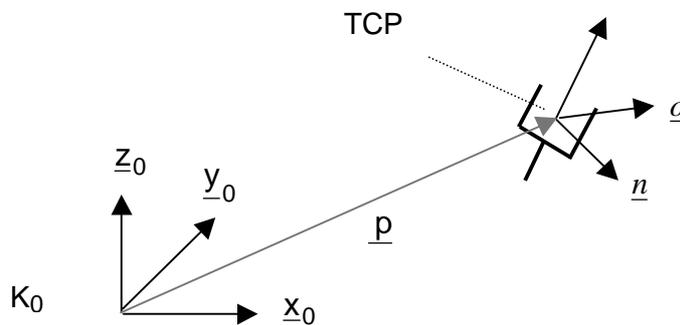
**Figure 2-2:** Description of the position and orientation of the tool center point (TCP) with respect to the base (world) frame  $K_0$
