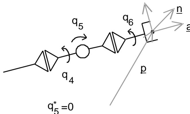
**Figure 3-3:** example for infinite solutions
