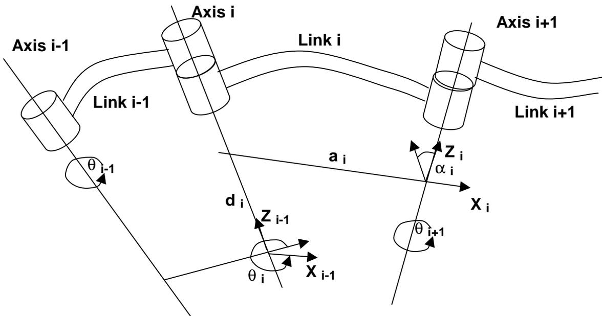
**Figure 3-2:** Link parameters  $\theta$ ,  $d$ ,  $a$  and  $\alpha$
