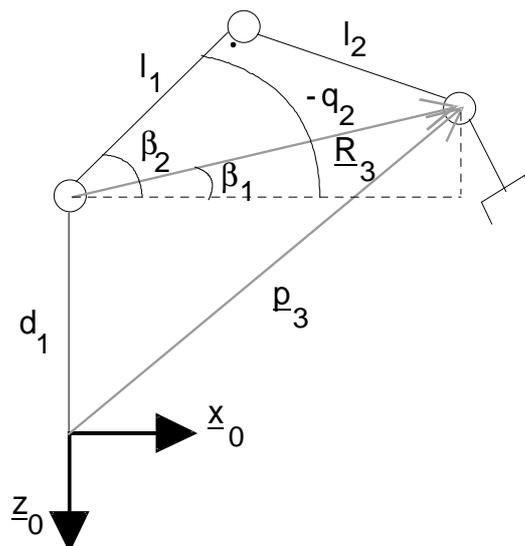
**Figure 3-6:** Calculation of  $q_2$
