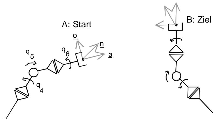
**Figure 4-1:** PTP motion between two points
