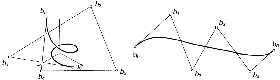
de Casteljau-Algorithm is used to calculate points on the Bezier curve:  $X_n(u_0)$
