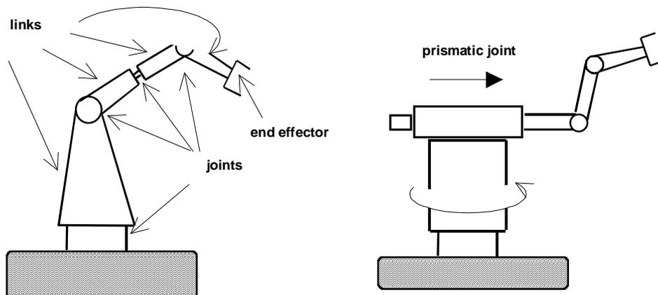
Industrial robots consist of (nearly) rigid links which are connected with **joints** which allow relative motion of neighboring **links**. These joints are usually instrumented with position sensors which allow the relative position of neighboring links to be measured. In case of rotary or **revolute** joints, these displacements are called joint angles. Some robots contain sliding, or **prismatic** joints.
