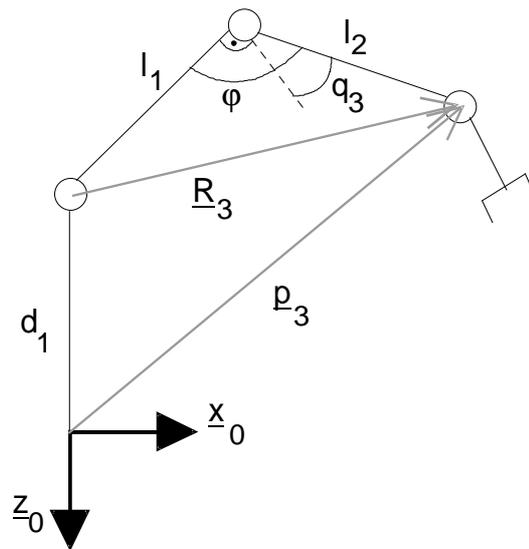
**Figure 3-5:** Calculation of  $q_3$
