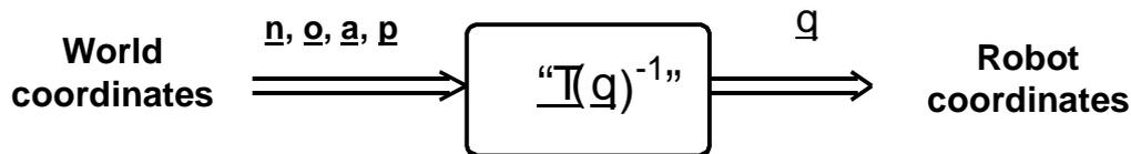
**Figure 3-1:** inverse kinematics: mapping from world coordinates to robot coordinates
