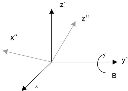
Angle C rotates around the new x-axis (x'')
