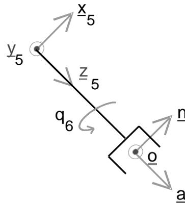
**Figure 3-9:** Calculation of  $q_6$
