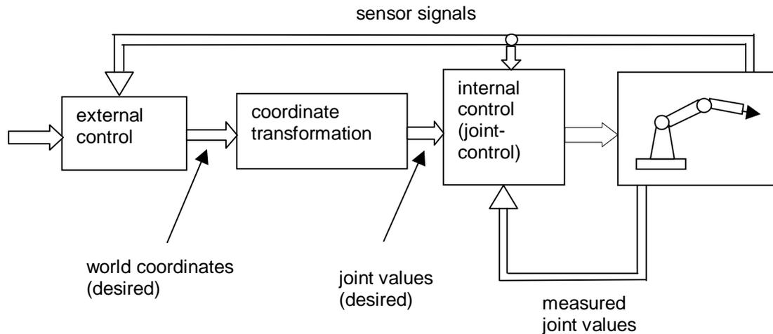
**Figure 1-1:** structure of a robot control
