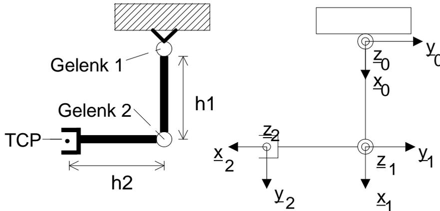
Figure 3-3: Planar 2-dof robot including coordinate system
